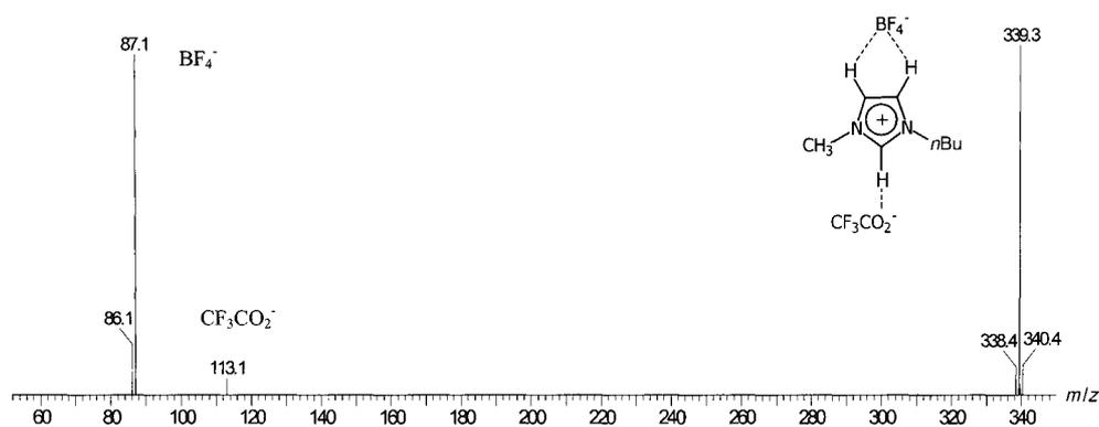
Figure 4. Tandem ESI-MS/MS product ion mass spectrum for 5 eV CID of the mixed and singly negatively charged ionic liquid supramolecule  $[\text{CF}_3\text{CO}_2\text{---X}_1\text{---BF}_4]^{-1}$ . The isotopologue ions  $^{11}\text{BF}_4^-$  of  $m/z$  87 and  $^{10}\text{BF}_4^-$  of  $m/z$  86 are lost preferentially since the hydrogen bond with  $\text{BF}_4^-$  is weaker than that with  $\text{CF}_3\text{CO}_2^-$ .
