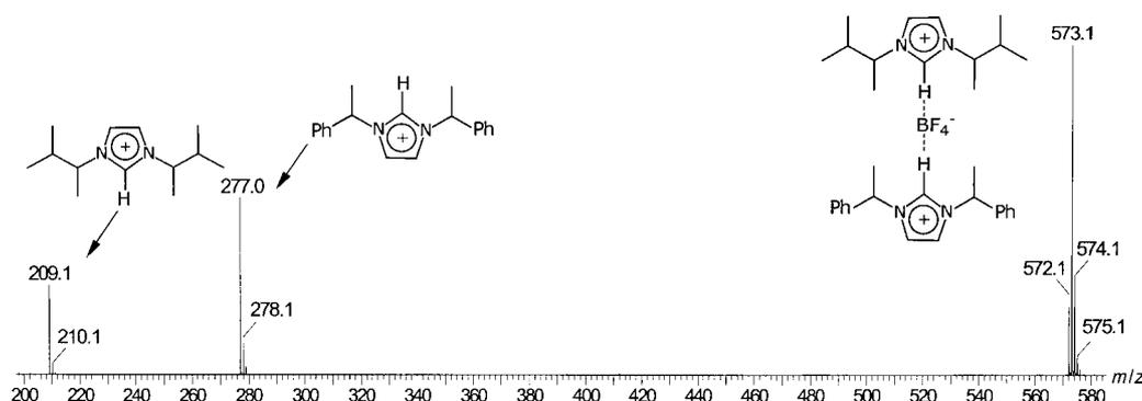
Figure 5. Tandem ESI-MS/MS product ion mass spectrum for 5 eV CID of the mixed and singly positively charged ionic liquid supramolecule  $[\text{X}^2\text{---BF}_4\text{---X}^3]^+$ . Because the H-bond of  $\text{X}^2$  of  $m/z$  209 to  $\text{BF}_4^-$  is stronger than that of  $\text{X}^3$ , the  $\text{X}^3$  fragment ion of  $m/z$  277 is formed to a greater extent.
