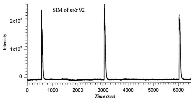
Figure 5. Headspace exposure FIMS profile for triplicate analysis (SIM of  $m/z$  92) of a 200 ppb toluene aqueous solution.
