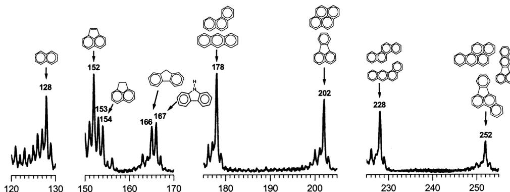
Figure 6. Collection of FIMS 70-eV EI mass spectra in the molecular ion region for a 1 ppb aqueous solution of a PAH mixture after variable fiber exposition times (5–30 min). Note that some isomeric PAHs are not distinguished by the mass spectrometric analysis.
