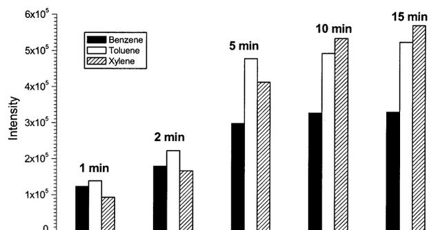
Figure 3. FIMS-SIM signal intensities for a 200 ppb BTX aqueous solution ( $m/z$  78 for benzene,  $m/z$  92 for toluene, and  $m/z$  106 for xylene) as a function of headspace fiber exposition time. Note that, on average, adsorption equilibrium is attained by 10 min.
