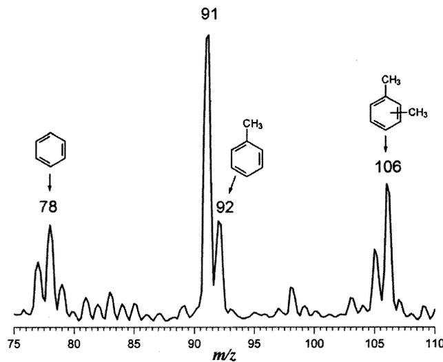
Figure 2. Partial 70-eV EI mass spectrum for a 100 ppb BTX aqueous solution acquired during the nearly 1-min desorption period of FIMS headspace analysis. Note the characteristic ions of  $m/z$  78 (benzene), 92 (toluene) and 106 (xylenes) and the considerably higher signal-to-noise ratio for full-scan single spectrum acquisition.
