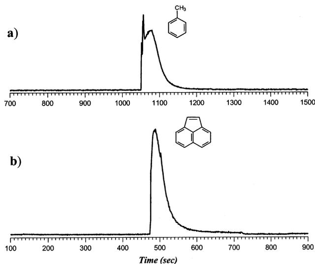
Figure 4. FIMS-SIM signal profile for aqueous solutions of (a) toluene (50 ppb) and (b) acenaphthylene (1 ppb) after 5 min of static headspace fiber exposure time for toluene and 30 min for acenaphthylene. Note the relatively narrow (nearly 1 min) and well-defined desorption peaks and the high signal-to-noise ratios.
