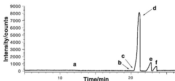
Fig. 2 Signal profile using SIM of  $m/z$  234 for the T&R-MIMS analysis of a 20  $\mu\text{M}$  aqueous Hcy solution after ECF derivatization.
