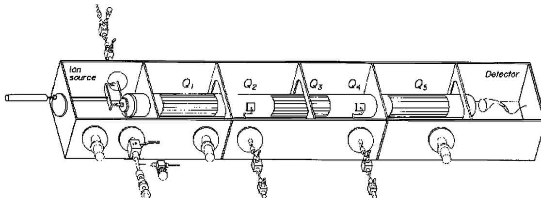
Fig. 2. Pentaquadrupole mass spectrometer and its arrangement of the three mass-analyzers ( $Q_1$ ,  $Q_3$  and  $Q_5$ ) and two “rf-only” quadrupole reaction chambers ( $Q_2$  and  $Q_4$ ).
