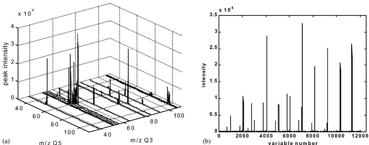
Fig. 4. (a) MS/MS spectrum from of 2-, 3- and 4-ethylpyridines (parent ion fragments  $m/z$  39, 51, 65, 79, 92, 106 and 107), with molar fraction 0.3/0.3/0.4, in the presence of deuterated pyridine (parent ion fragments  $m/z$  52, 54, 56 and 84); (b) unfolding spectrum, where in the abscissa is plotted the number of points.
