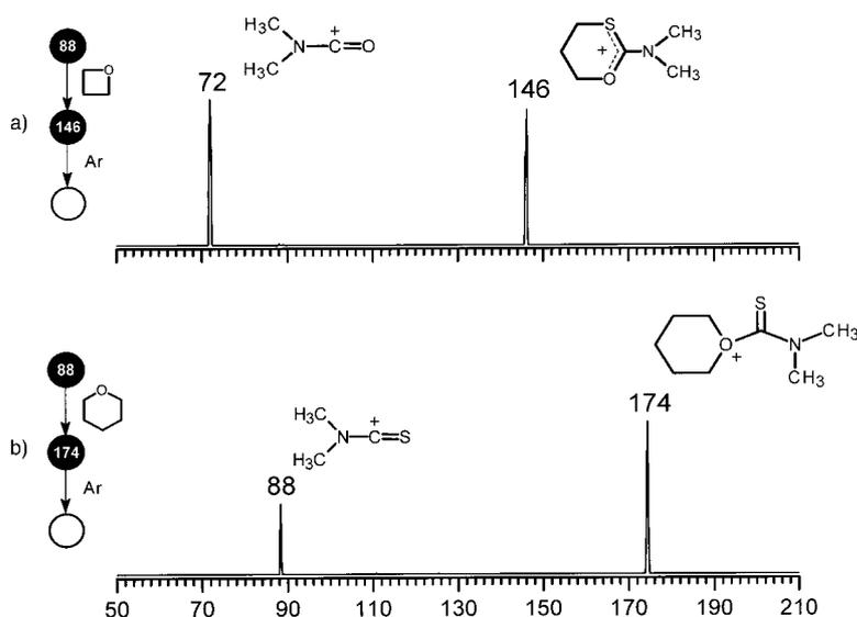
Figure 5. Triple-stage ( $MS^3$ ) sequential product ion mass spectra for the adducts formed in reactions of  $(CH_3)_2N-C=S$  with: a) tetramethylene oxide and b) tetrahydropyran.
