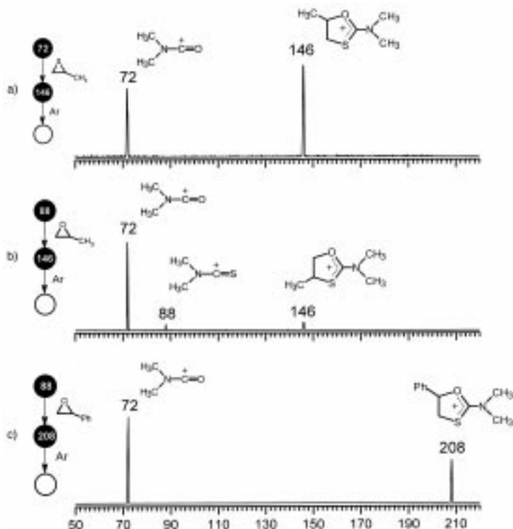
Figure 2. Triple-stage ( $MS^3$ ) sequential product ion mass spectra for the adducts formed in reactions of: a)  $(\text{CH}_3)_2\text{N}-\text{C}^+=\text{O}$  with propylene sulfide; b)  $(\text{CH}_3)_2\text{N}-\text{C}^+=\text{S}$  with propylene oxide; and c)  $(\text{CH}_3)_2\text{N}-\text{C}^+=\text{S}$  with styrene oxide.
