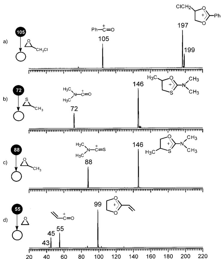
Figure 1. Double-stage ( $MS^2$ ) product ion mass spectra for reactions: a)  $\text{Ph}-\text{C}^+=\text{O}$  of  $m/z$  105 with epichlorohydrin; b)  $(\text{CH}_3)_2\text{N}-\text{C}^+=\text{O}$  of  $m/z$  72 with propylene sulfide; c)  $(\text{CH}_3)_2\text{N}-\text{C}^+=\text{S}$  of  $m/z$  88 with propylene oxide; and d)  $\text{CH}_2=\text{CH}-\text{C}^+=\text{O}$  of  $m/z$  55 with ethylene oxide.
