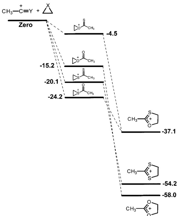
Figure 8. Ab initio MP2/6–311G(d,p)//HF/6–311G(d,p) + ZPE potential energy surface diagram for the three-to-five ring-expansion Meerwein reaction of  $\text{CH}_3-\overset{\oplus}{\text{C}}=\text{O}$  or  $\text{CH}_3-\overset{\oplus}{\text{C}}=\text{S}$  with ethylene oxide ( $\text{X}=\text{O}$ ) or ethylene sulfide ( $\text{X}=\text{S}$ ). Reaction barriers were not estimated, and are not indicated.
