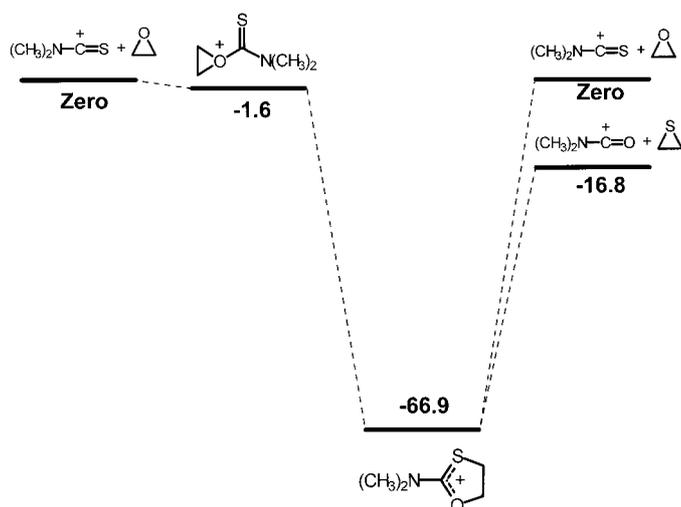
Figure 7. Ab initio MP2/6–311G(d,p)//HF/6–311G(d,p) + ZPE potential energy surface diagram for the gas-phase Meerwein reaction of  $(\text{CH}_3)_2\text{N}-\overset{\oplus}{\text{C}}=\text{S}$  with ethylene oxide and the dissociation thresholds of the 1,3-oxathiolanylium ion. Reaction barriers were not estimated, and are not indicated.
