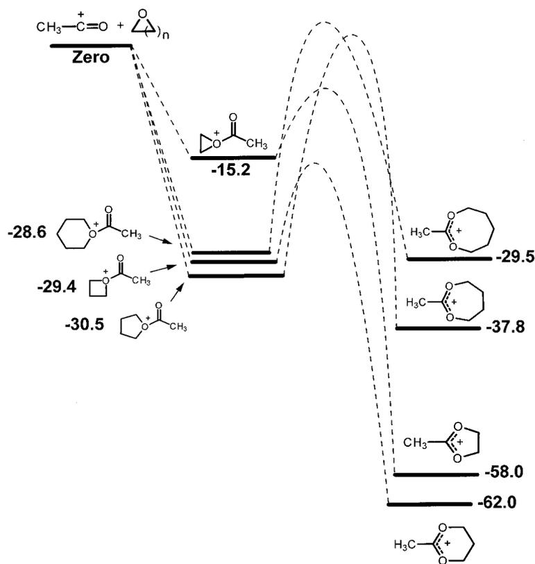
Figure 9. Ab initio MP2/6-311G(d,p)//HF/6-311G(d,p) + ZPE potential energy surface diagram for four-to-six-membered ring-expansion on reactions of  $\text{CH}_3\text{-CO}^+$  with ethylene oxide or trimethylene oxide, tetrahydrofuran, and tetrahydropyran. Reaction barriers were not estimated, but expected trends in activation energies are indicated.
