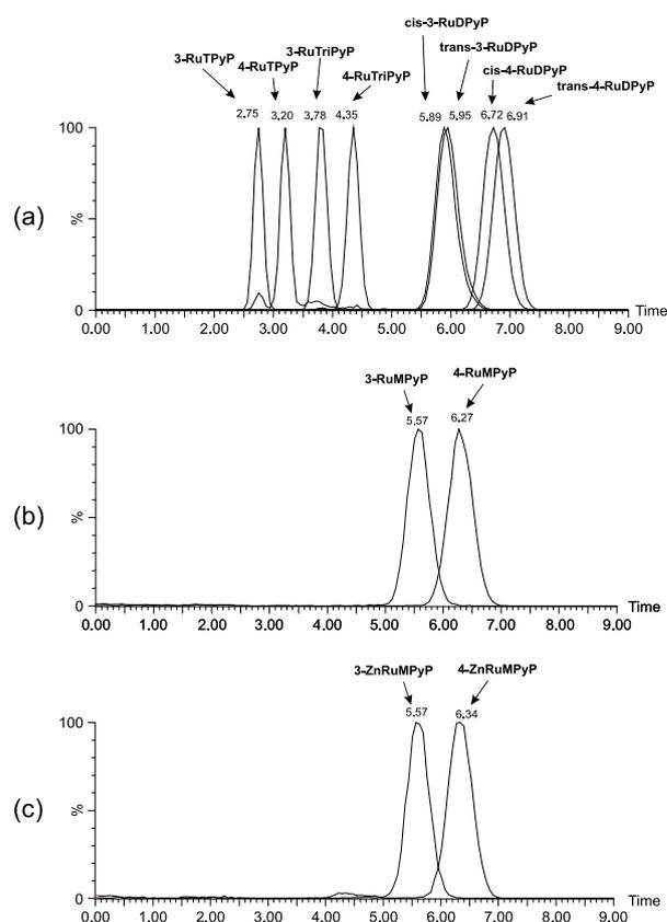
**Figure 3.** Overlaid drift time plots for (a) **3-RuTPyP**, **4-RuTPyP**, **3-RuTriPyP**, **4-RuTriPyP**, *cis*-**3-RuDPyP**, *cis*-**4-RuDPyP**, *trans*-**3-RuDPyP** and *trans*-**4-RuDPyP** (wave parameters: 300 m/s, 27.0 V), (b) **3-RuMPyP** and **4-RuMPyP** (wave parameters: 182 m/s, 30.0 V), and (c) **3-ZnRuMPyP** and **4-ZnRuMPyP** (wave parameters: 182 m/s, 30.0 V) using  $CO_2$  at 1 mbar of pressure as drift gas.
