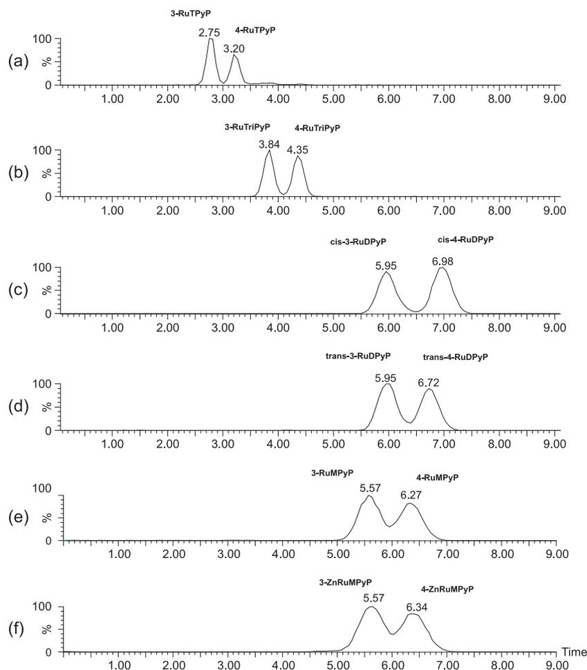
**Figure 4.** Drift time plots for mixtures of (a) 3-RuTPyP and 4-RuTPyP, (b) 3-RuTriPyP and 4-RuTriPyP, (c) *cis*-3-RuDPyP and *cis*-4-RuDPyP, (d) *trans*-3-RuDPyP and *trans*-4-RuDPyP, (e) 3-RuMPyP and 4-RuMPyP, and (f) 3-ZnRuMPyP and 4-ZnRuMyP, using CO<sub>2</sub> at 1 mbar. (a)-(d) wave velocity 300 m/s and wave height 27 V; (e)-(f) wave velocity 182 m/s and wave height 30 V.
