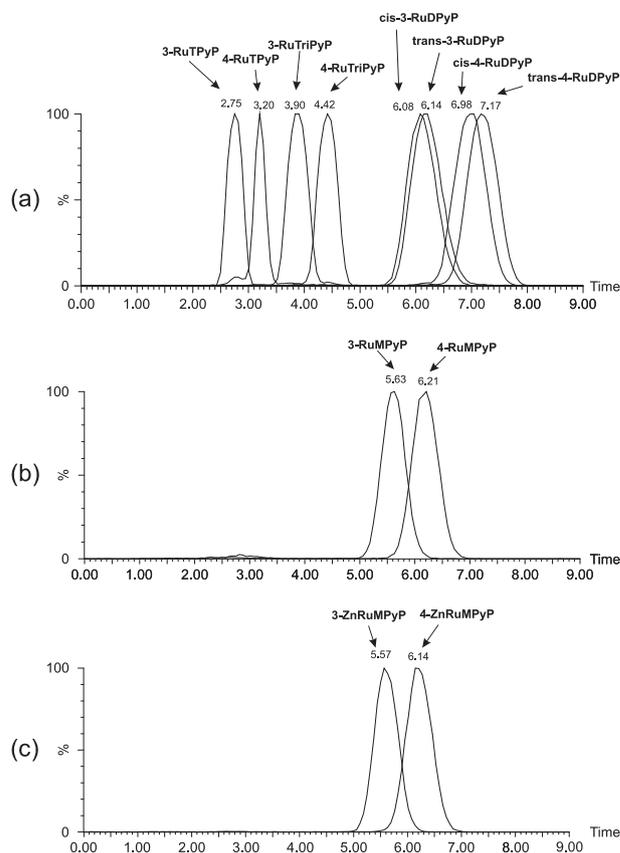
**Figure 1.** Overlaid drift time plots for (a) **3-RuTPyP**, **4-RuTPyP**, **3-RuTriPyP**, **4-RuTriPyP**, **cis-3-RuDPyP**, **cis-4-RuDPyP**, **trans-3-RuDPyP** and **trans-4-RuDPyP** (wave parameters: 300 m/s, 13.6 V), (b) **3-RuMPyP** and **4-RuMPyP** (wave parameters: 300 m/s, 22.0 V), and (c) **3-ZnRuMPyP** and **4-ZnRuMPyP** (wave parameters: 300 m/s, 22.0 V) using N<sub>2</sub> at 1 mbar of pressure as drift gas.
