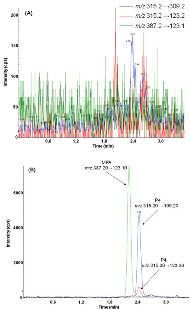
Fig. 2. Chromatograms showing the selectivity of the liquid chromatography coupled to tandem mass spectrometry (LC-MS/MS) method for progesterone (P<sub>4</sub>) quantitation. (A) A blank plasma extraction and (B) a plasma extract that contains P<sub>4</sub> and medroxyprogesterone 17-acetate (MPA) at the limit of quantitation (LOQ) are represented.
