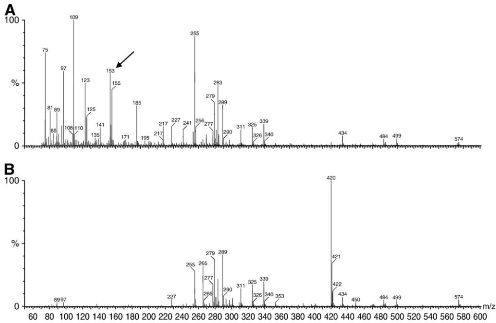
Fig. 4. ESI(–)-MS of apple juice (A) contaminated and (B) uncontaminated with patulin. The contaminated juice was inoculated with *B. fulva* IOC 4518 ( $10^3$  spores/mL).
