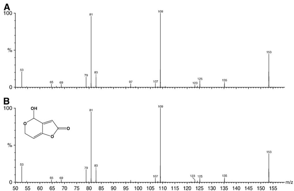
Fig. 5. ESI(–)-MS/MS of the ion of  $m/z$  153 from A) the contaminated juice and B) from a patulin standard.
