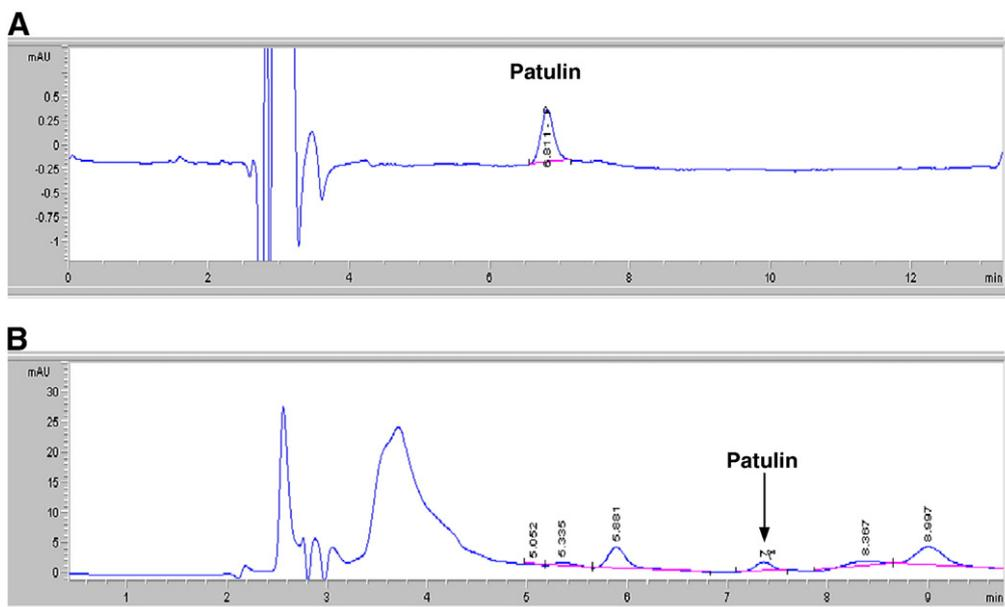
Fig. 3. HPLC chromatograms showing the characteristic peak of patulin as detected using a UV detector ( $\lambda = 276$  nm). (A) Peak refers to the standard solution (apple juice) spiked with 0.5 µg/kg of patulin; (B) peak refers to the patulin quantified in apple juice (211 µg/kg) inoculated with *B. fulva* IOC 4518 and incubated for 14 days at 30 °C.
