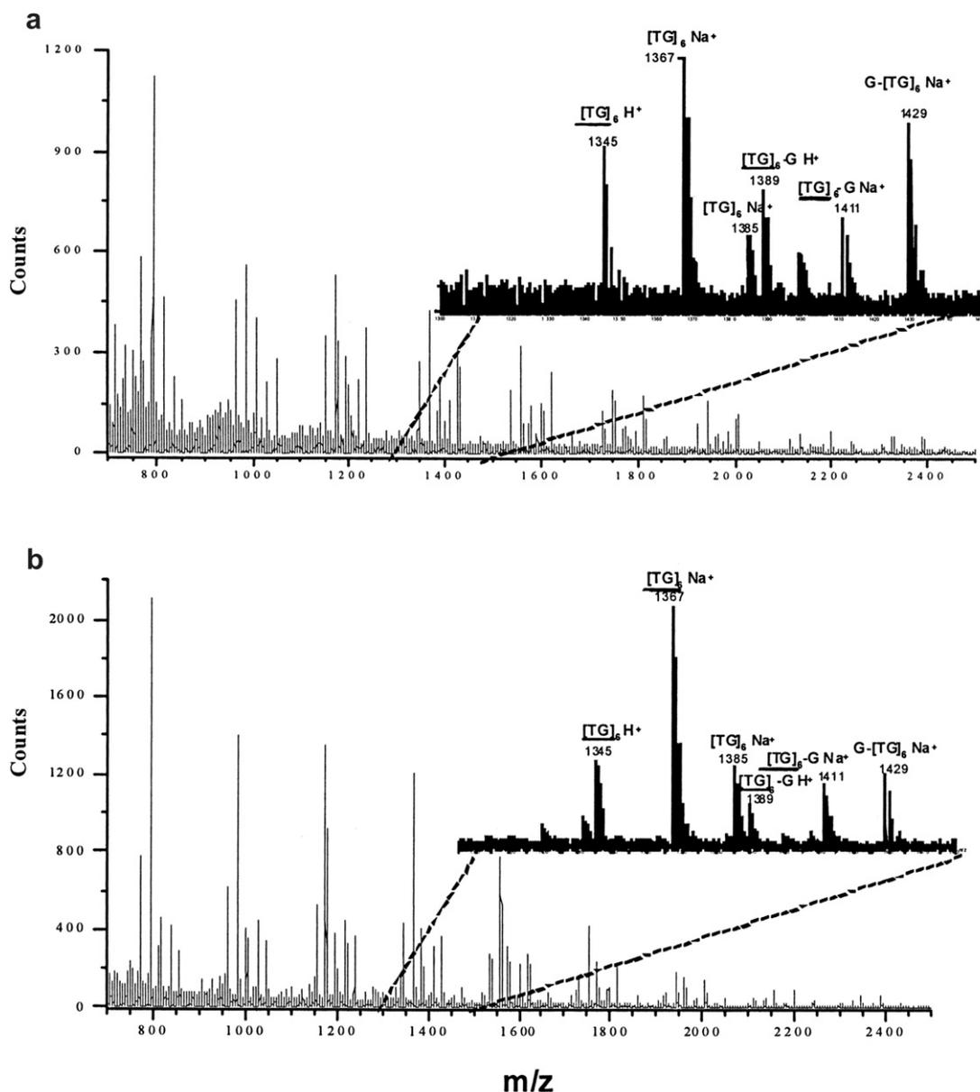
**Fig. 1.** MALDI-MS of oligomers extracted from (a) virgin bottle-grade PET resin (PET<sub>v</sub>-btg I) and (b) PET from post-consumed soft-drink bottles (PET<sub>pc</sub>-btg), processed using a counter-rotating twin-rotors mixer at 250 °C, 50 rpm for 5 min. The inserts show an expanded view of the spectra in the *m/z* range of 1300–1450.
