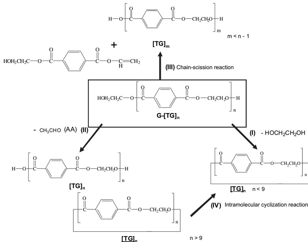
**Fig. 2.** Oligomers extracted from PET and detected by MALDI-MS and the mechanism for their formation via thermomechanical degradation.
