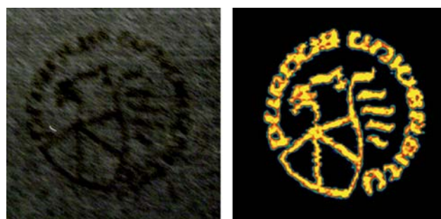
Fig. 8 (Left) An “invisible stamp” simulated by using black ink and black paper and (right) the image resulting from diagnostic ion-selective development by 2D DESI-MS imaging.
