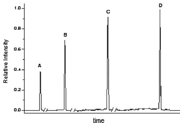
**Figure 2.** T&R-MIMS responses using SIM ( $m/z$  94) for the analysis of a  $1000 \mu\text{g L}^{-1}$  acetylated phenol aqueous solution as a function of trapping time: (A) 5, (B) 10, (C) 15, and (D) 20 min. For optimum sensitivity and analytical frequency, a trapping time of 15 min (C) was selected. An air plug of 1 min was used, based on previous testing of the system.<sup>18</sup>
