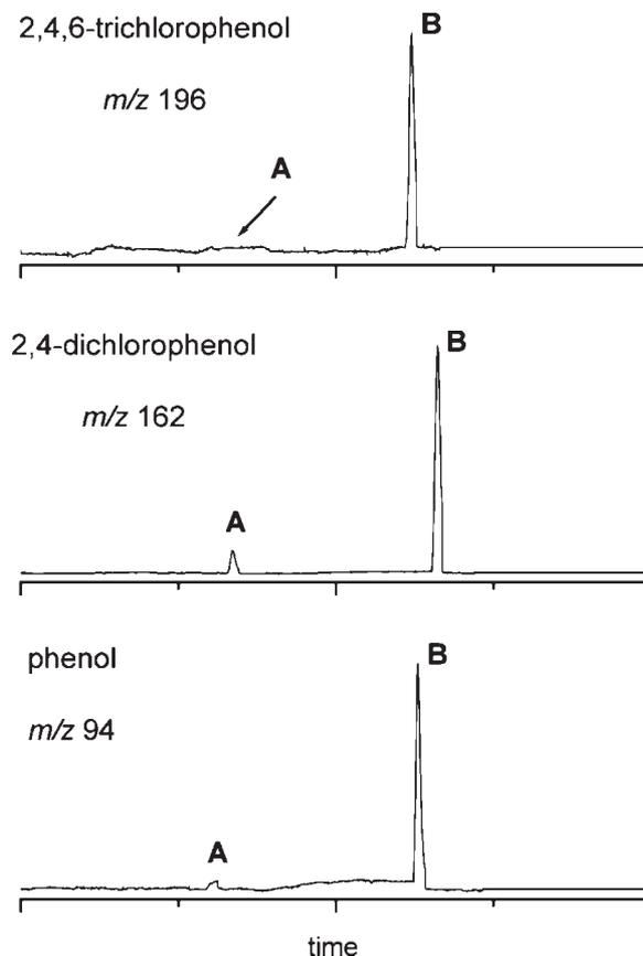
**Figure 3.** T&R-MIMS responses using SIM for the analysis of a  $1000 \mu\text{g L}^{-1}$  phenol aqueous solution after 15 min of trapping and 1 min air plug (A) without and (B) with acetylation.
