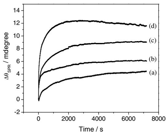
Fig. 8. Adsorption of  $\beta$ CDSH from ethanol on gold at different concentrations: (a)  $1 \mu\text{mol l}^{-1}$ , (b)  $10 \mu\text{mol l}^{-1}$ , (c)  $100 \mu\text{mol l}^{-1}$ , (d)  $500 \mu\text{mol l}^{-1}$ .
