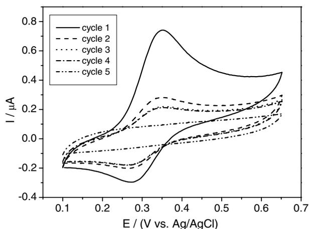
Fig. 12. Cyclic voltammograms obtained after the pre-concentration of  $\text{FeCO}_2\text{H}$  on  $\beta\text{CDSH}$  monolayer taken in a  $\text{KCl}$   $0.1 \text{ mol l}^{-1}$  solution from first up to fourth cycle of potential (cycle 1 up to cycle 4). Cycle 5 become referring to the cyclic voltammogram to modified electrode after the carried cycle 4 in a supporting electrolyte solution without  $\text{FeCO}_2\text{H}$  molecules.
