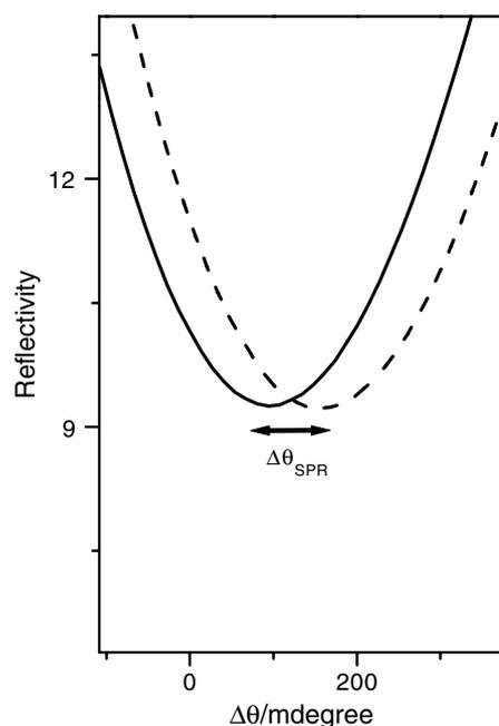
Fig. 3. SPR reflectivity curves for a clean gold surface in ethanol (solid line) and the same surface after the adsorption of  $\beta$ CDSH in ethanol solution (dashed line).
