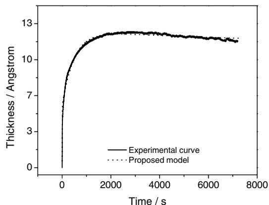
Fig. 7. Adsorption of mono(6-deoxy-6-mercapto)- $\beta$ -cyclodextrin from an ethanol solution of  $500 \mu\text{mol l}^{-1}$  of the thiol (solid line). The dot line represents the curve calculated from rearrange-limited Langmuir model.
