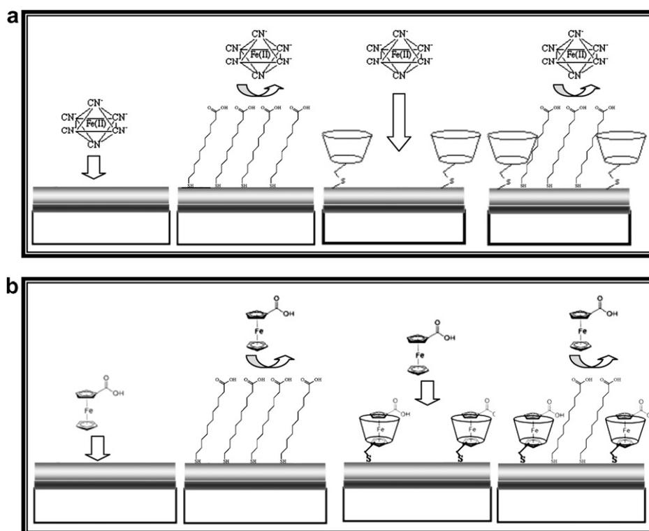
Fig. 10. Schematic diagram referring to the  $[\text{Fe}(\text{CN})_6]^{3-}$  (a) and ferrocenemonocarboxylic acid (b) interaction with: (1) bare electrode, (2) MUA monolayer, (3)  $\beta$ CDSH monolayer and (4) mixed MUA/ $\beta$ CDSH monolayer.
