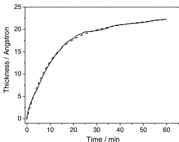
Fig. 5. Adsorption of mono(6-deoxy-6-mercapto)- $\beta$ -cyclodextrin from a  $500 \mu\text{mol l}^{-1}$  thiol ethanolic solution under hydrostatic conditions (solid line). The dashed line represents the curve calculated from the multilayer model which well adjusts to the experimental curve resulting in a non-linear regression coefficient of 0.9938 and a also a non-linear chi-square of 0.0208.
