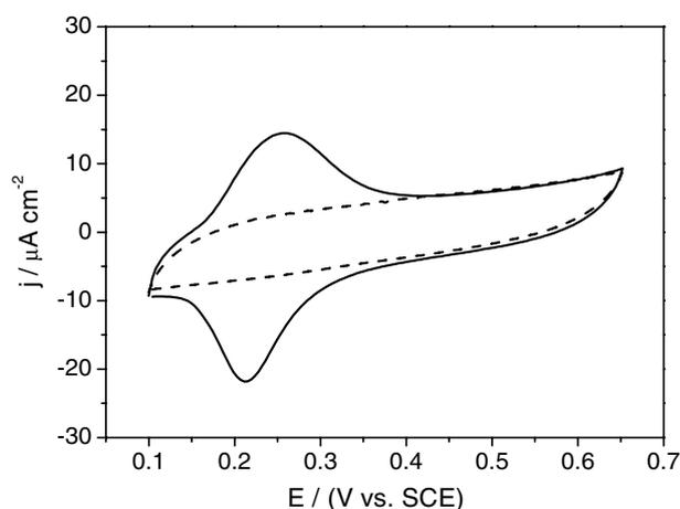
Fig. 11. Pre-concentration of  $\text{FeCO}_2\text{H}$  on mixed MUA/ $\beta$ CDSH monolayer (full line) and the same experiment on MUA monolayer (dashed line).
