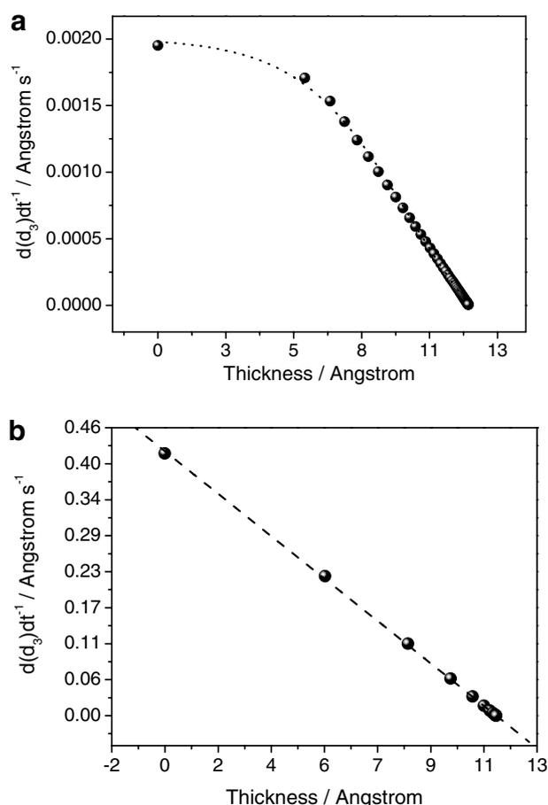
Fig. 6. Lines obtained from the association phase of Fig. 5 transformed into plots of  $d(d_3)dt^{-1}$  versus  $d_3$ : (a) non-flow and (b) flow rate  $30 \mu\text{l s}^{-1}$ .
