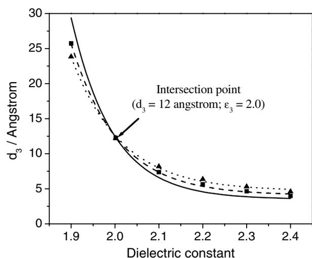
Fig. 4. Dielectric constants and thickness of the mono(6-deoxy-6-mercapto)- $\beta$ -cyclodextrin film obtained from SPR spectra. Each curve represents a series of film thickness and dielectric constants when the ethanol (solid line), and the binary ethanol/deionized water (75/25 dashed line) and (50/50 dotted line) were used.
