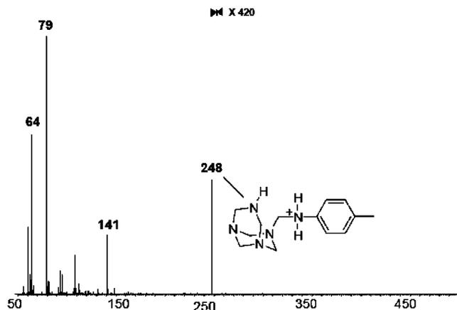
**FIGURE 5.** ESI-MS screening for the reaction solution formed by mixing TFA solutions of *p*-toluidine (**1**) with urotropine (**15**) on-line using a microreactor coupled just before the ESI source and reaction time of ca. 2.0 s and not 0.7 s.
