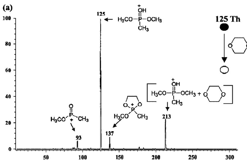
**Figure 15.** Product ion mass spectra for the reaction of the phosphonium ion  $\text{CH}_3\text{OP}(\text{O})\text{CH}_3^+$  of  $m/z$  93 formed by methanol loss from protonated dimethyl methylphosphonate (DMMP) of  $m/z$  125. Adapted from Ref. 44.
