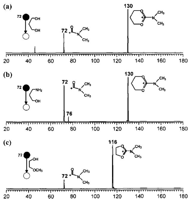
**Figure 11.** Product ion mass spectra for reactions of the acylium ion  $(\text{CH}_3)_2\text{NCO}^+$  of  $m/z$  72 with (a) 1,3-propanediol, (b) 3-amino-1-propanol and (c) 2-methoxyethanol. Adapted from Ref. 28.
