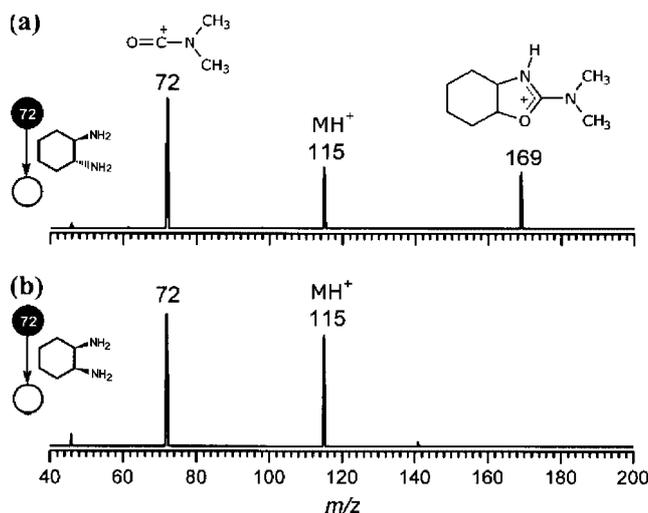
**Figure 12.** Product ion mass spectra for the reaction of the acylium ion  $(\text{CH}_3)_2\text{N}-\text{C}^+=\text{O}$  of  $m/z$  72 with the stereoisomeric pair of (a) *trans*- and (b) *cis*-diamine cyclohexane. Adapted from Ref. 36.
