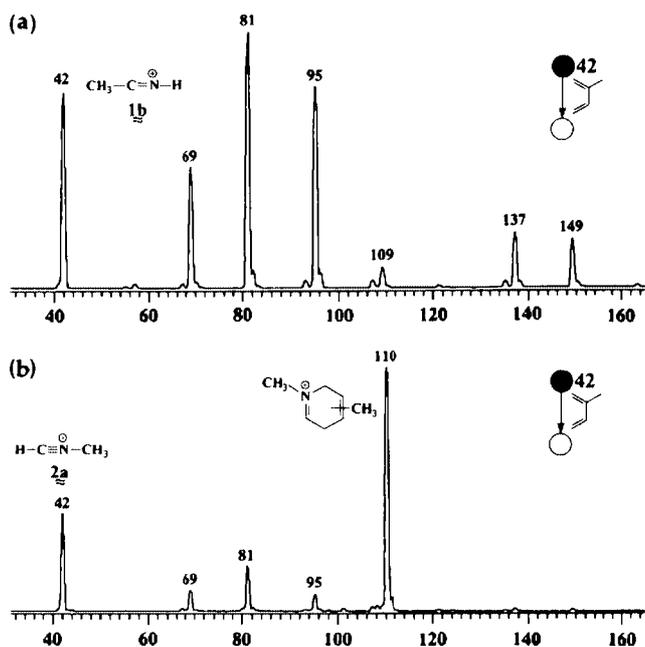
**Figure 3.** Product ion mass spectra for the reactions of the isomeric ions and (a) CH<sub>3</sub>-C≡N<sup>+</sup>-H and (b) H-C≡N<sup>+</sup>-CH<sub>3</sub> of *m/z* 42 with isoprene. Adapted from Ref. 26.
