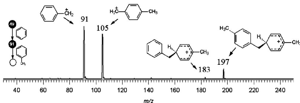
**Figure 8.** Sequential product ion mass spectrum for the reactions of the benzylum ion of  $m/z$  91 (formed via reactions of  $CH_2^{35}Cl^+$  of  $m/z$  49 with benzene) with toluene. Adapted from Ref. 32.
