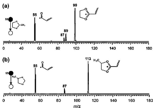
**Figure 14.** Product ion mass spectra for the reaction of the acylium ion  $\text{CH}_2=\text{CH}-\text{C}^+=\text{O}$  of  $m/z$  55 with two isomeric acetals. Adapted from Ref. 41.
