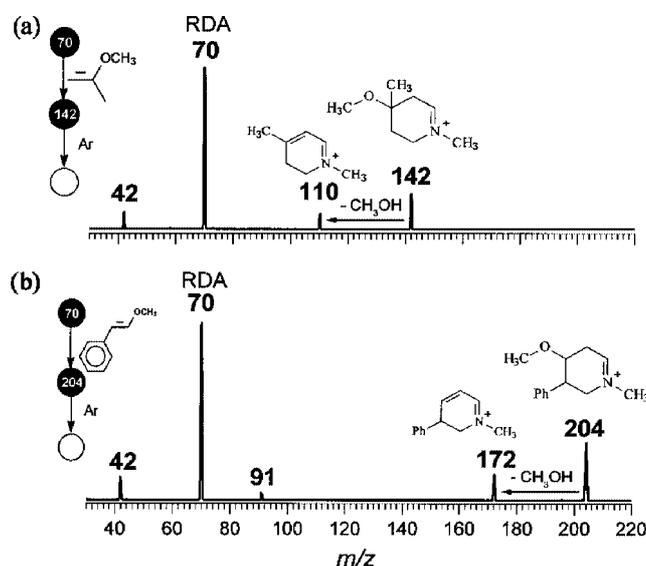
**Figure 6.** Sequential product ion mass spectrum for the  $[4^+ + 2]$  cycloadduct of  $\text{MAB}^+$  with (a) 2-propenyl vinyl ether ( $m/z$  142) and (b)  $\beta$ -methoxy styrene ( $m/z$  204). Adapted from Ref. 28.
