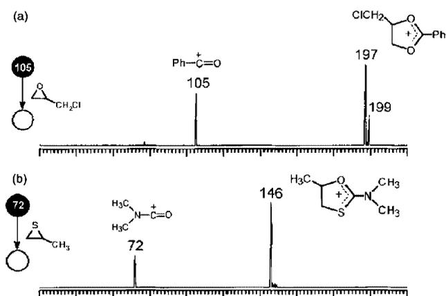
**Figure 2.** Product ion mass spectra for the reactions of (a) Ph-C<sup>+</sup>=O with epichlorhydrin and (b) of (CH<sub>3</sub>)<sub>2</sub>N-C<sup>+</sup>=O with propylene sulfide. Adapted from Ref. 20.
