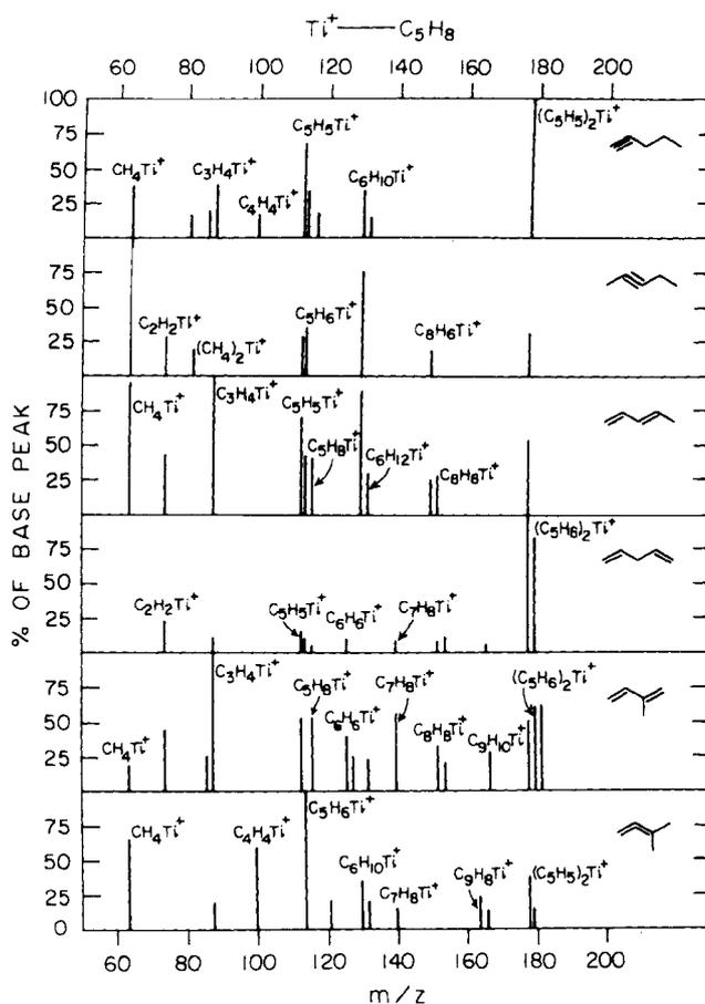
**Figure 22.** Product ion ( $\text{MS}^2$ ) mass spectra for the reaction of  $\text{Ti}^+$  with several  $\text{C}_5\text{H}_8$  isomeric molecules. Adapted from Ref. 59.
