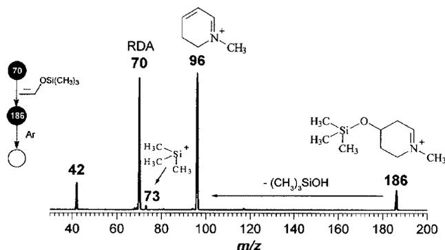
**Figure 5.** Sequential product ion mass spectrum for the  $[4^+ + 2]$  cycloadduct of  $m/z$  186 formed via reactions of  $\text{MAB}^+$  with vinyloxy trimethylsilane. Adapted from Ref. 28.
