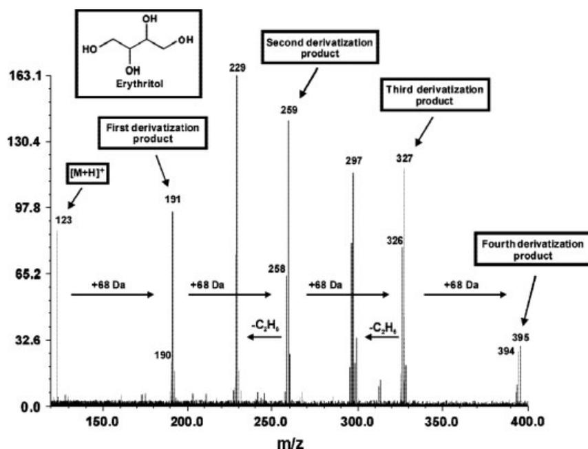
**Figure 18.** Product ion mass spectrum for the reaction of protonated erythritol (a tetrol) with diethylmethoxyborane. Adapted from Ref. 51.
