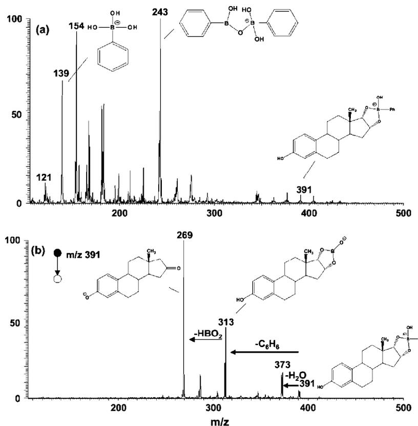
**Figure 23.** (a) DESI mass spectrum showing the products of on-surface ambient reactions of  $\text{PhB(OH)}_3^-$  anion with *cis*-estriol; (b) Product ion mass spectrum of the reaction product ion of *cis*-estriol of  $m/z$  391. Adapted from Ref. 64.
