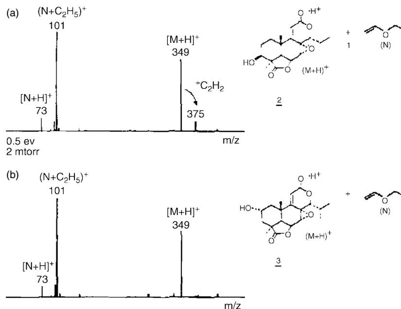
**Figure 9.** Product ion mass spectra for the reactions of an isomeric pair of protonated (a)  $\beta$ - and (b)  $\gamma$ -hydroxycarbonyl compounds with ethyl vinyl ether (N). The class-selective product is that of  $m/z$  375. The ion of  $m/z$  101 arises from ethylation of N by  $[N+H]^+$ . Adapted from Ref. 33.
