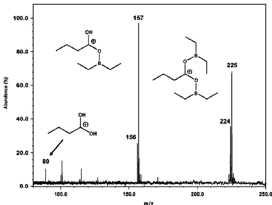
Figure 19. Product ion ( $\text{MS}^2$ ) mass spectrum for the reaction of protonated butanoic acid with diethyl methoxyborane. Adapted from Ref. 39.
