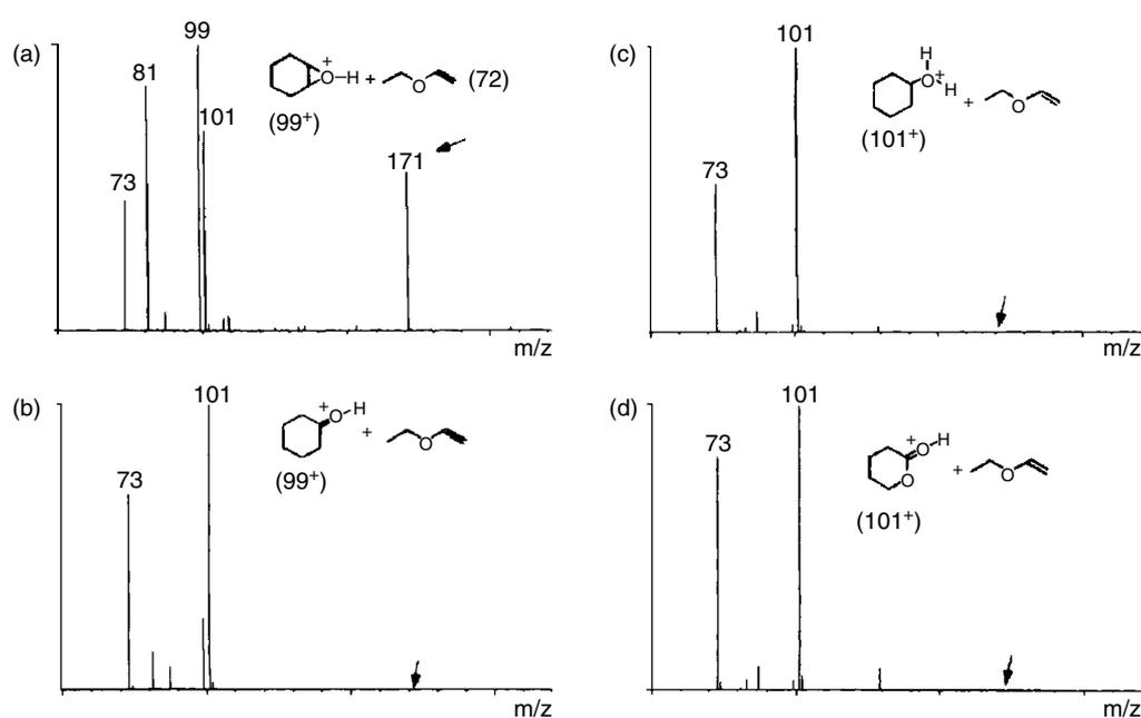
**Figure 1.** Product ion mass spectra for the reactions with ethyl vinyl ether of protonated molecules of (a) cyclohexene oxide (b) cyclohexanone (c) cyclohexanol and (d)  $\gamma$ -valerolactone. Adapted from Ref. 19.
