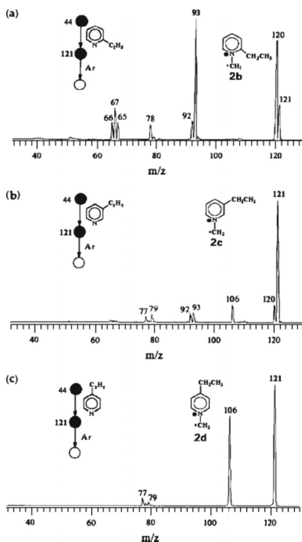
**Figure 16.** Sequential product ion mass spectra for the product ions of  $m/z$  121 formed by  $\text{CH}_2^+\bullet$  transfer from  $^{\bullet}\text{CH}_2-\text{O}-\text{CH}_2^+$  to isomeric ethyl pyridines. Adapted from Ref. 45.
