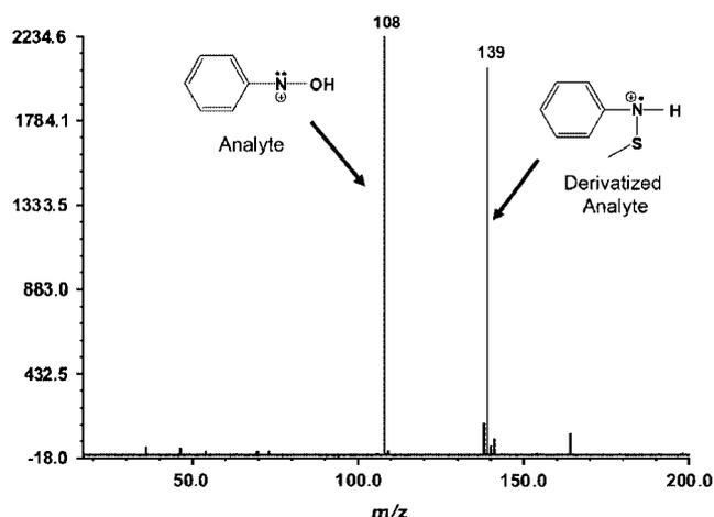
**Figure 21.** Product ion ( $\text{MS}^2$ ) mass spectra for the reaction of protonated nitrosobenzene with dimethyl disulfide. Adapted from Ref. 55.
