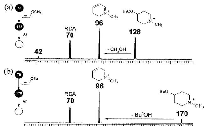
**Figure 4.** Sequential product ion mass spectrum for the  $[4^+ + 2]$  cycloadduct of  $\text{MAB}^+$  with (a) methyl vinyl ether of  $m/z$  128 and (b) *n*-butyl vinyl ether of  $m/z$  170. Adapted from Ref. 28.
