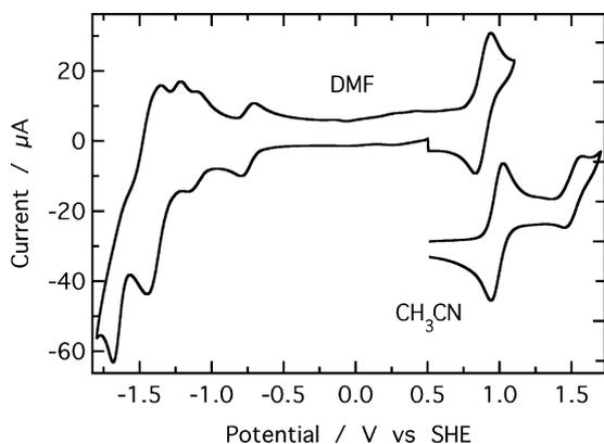
Fig. 7. Cyclic voltammogram of a  $2.0 \times 10^{-3}$  M solution of  $H_2(3\text{-TRPyP})$  in DMF,  $100 \text{ mV s}^{-1}$ . Inset: Cyclic voltammogram of a  $2.0 \times 10^{-3}$  M solution in  $\text{CH}_3\text{CN}$ , in the 0.50 to 1.65 V range and DPV results for the Ru(III/II) and Porph(-1/0) process.
