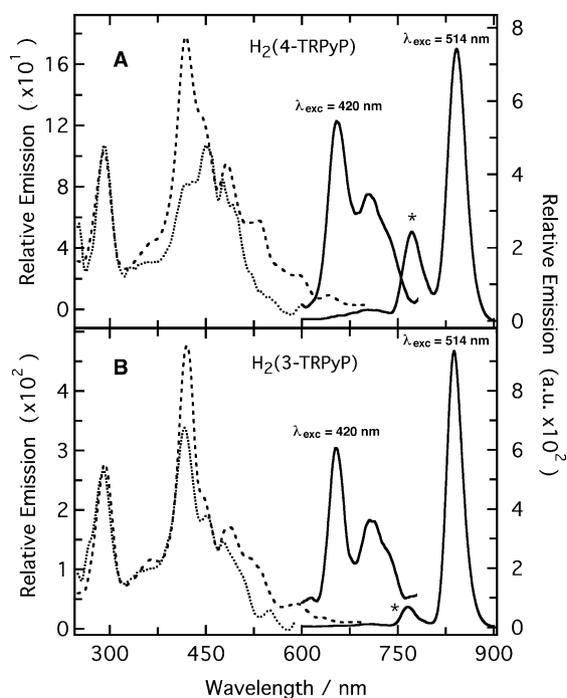
Fig. 6. Luminescent emission (right axis;  $\lambda_{\text{exc}} = 420$  and  $514 \text{ nm}$ ) and excitation spectra (left axis;  $\lambda_{\text{em}} = 655$  (dashed line) and  $840 \text{ nm}$  (dotted line)) of (A)  $\text{H}_2(4\text{-TRPyP})$  and (B)  $\text{H}_2(3\text{-TRPyP})$  supermolecules, in ethanol glass, at  $77 \text{ K}$ . \* scattering.
