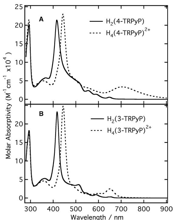
Fig. 5. UV-Vis spectra of  $\sim 3.0 \mu\text{M}$  solutions of protonated (dashed lines) and non-protonated (solid lines) (A)  $\text{H}_2(4\text{-TRPyP})$  and (B)  $\text{H}_2(3\text{-TRPyP})$ , in methanol. The protonation was carried out by dissolving gaseous HCl into the solution.
