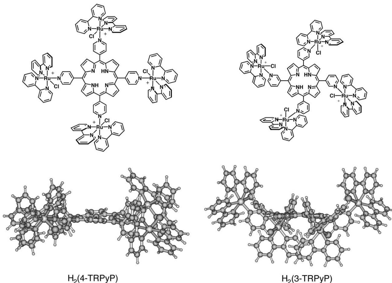
Fig. 1. Schematic and respective lateral view of the geometry optimized structures of the  $H_2(4\text{-TRPyP})$  and  $H_2(3\text{-TRPyP})$  complexes.
