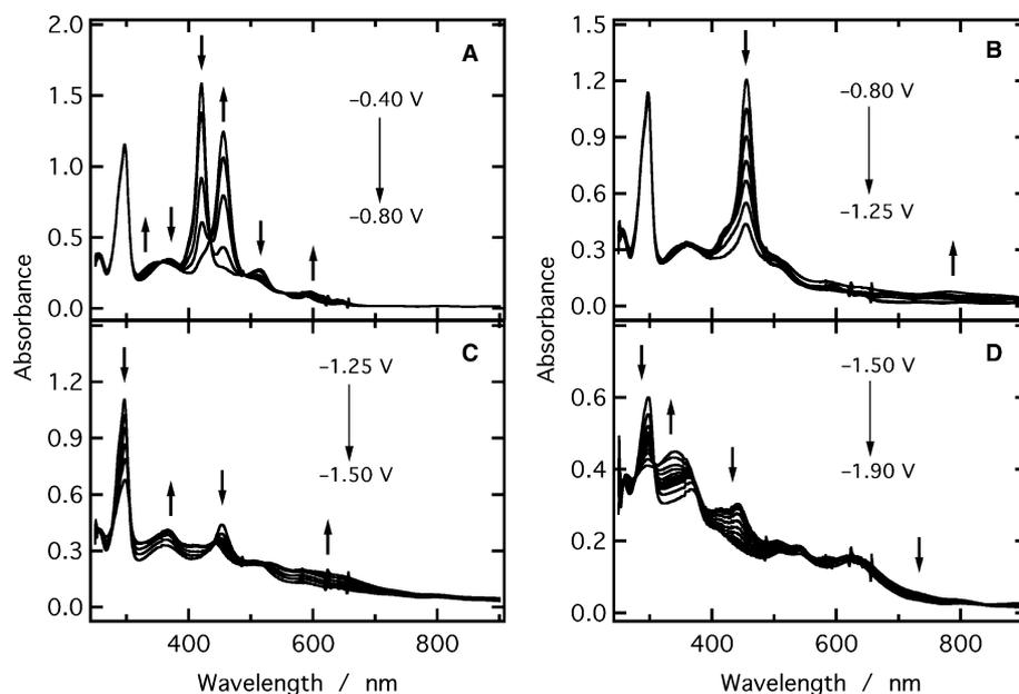
Fig. 9. Spectroelectrochemistry of  $1.5 \times 10^{-3}$  M  $\text{H}_2(3\text{-TRPyP})$  in the (A)  $-0.40$  to  $-0.80$  V, (B)  $-0.80$  to  $-1.25$  V, (C)  $-1.25$  to  $-1.50$  V and (D)  $-1.50$  to  $-1.90$  V range. Electrolyte:  $0.10$  M  $\text{TEAClO}_4$  in DMF.
