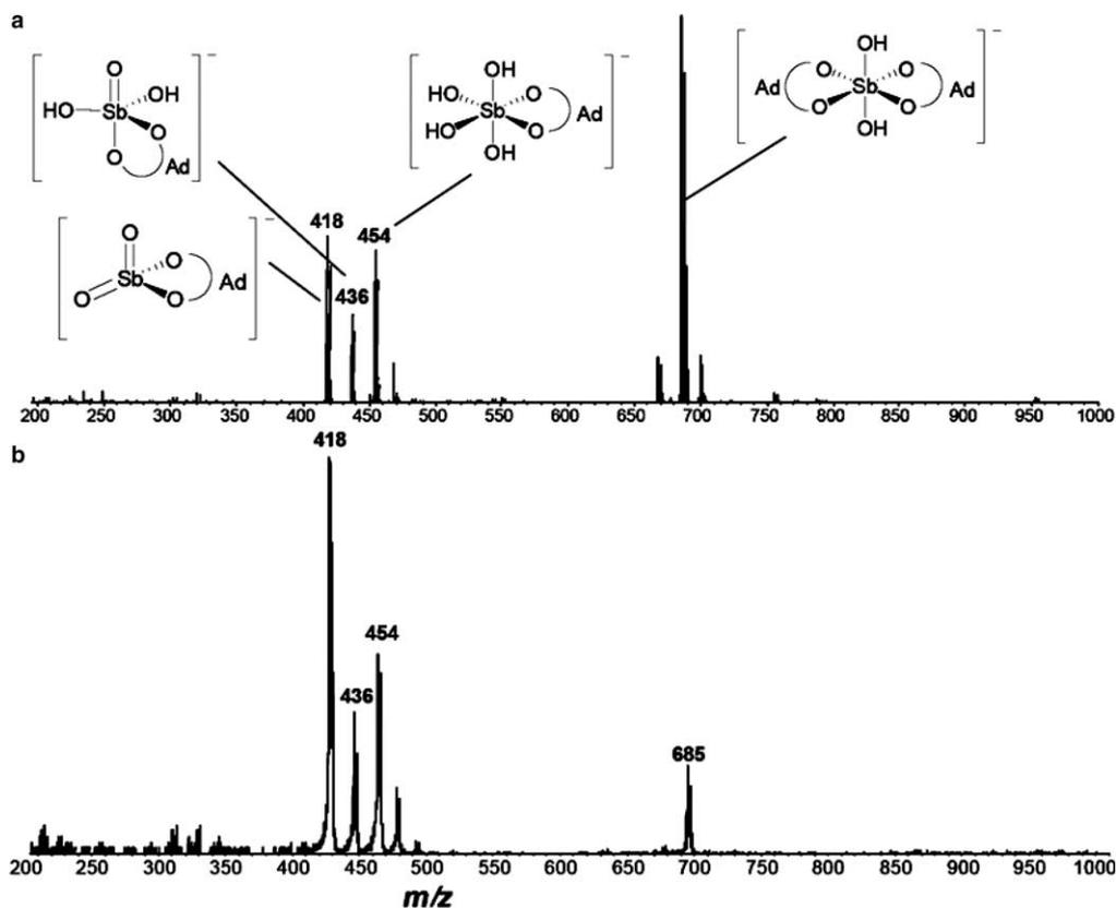
Fig. 1. ESI(–) mass spectra for water/methanol solutions of the Sb–adenosine (Ad) complexes: (a) **a** and (b) **b**. The proton source for the deprotonated species are not indicated.
