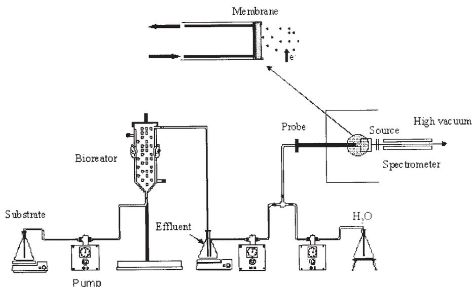
**Figure 1.** A schematic representation of the bioreduction-MIMS instrumental set-up.
