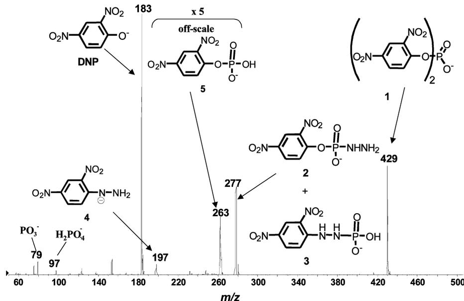
**FIGURE 3.** Typical ESI-MS mass spectra of the reaction mixture of 0.01 M BDNPP with 0.1 M NH<sub>2</sub>NH<sub>2</sub> in aqueous methanol (50% v/v) at pH 4–7.
