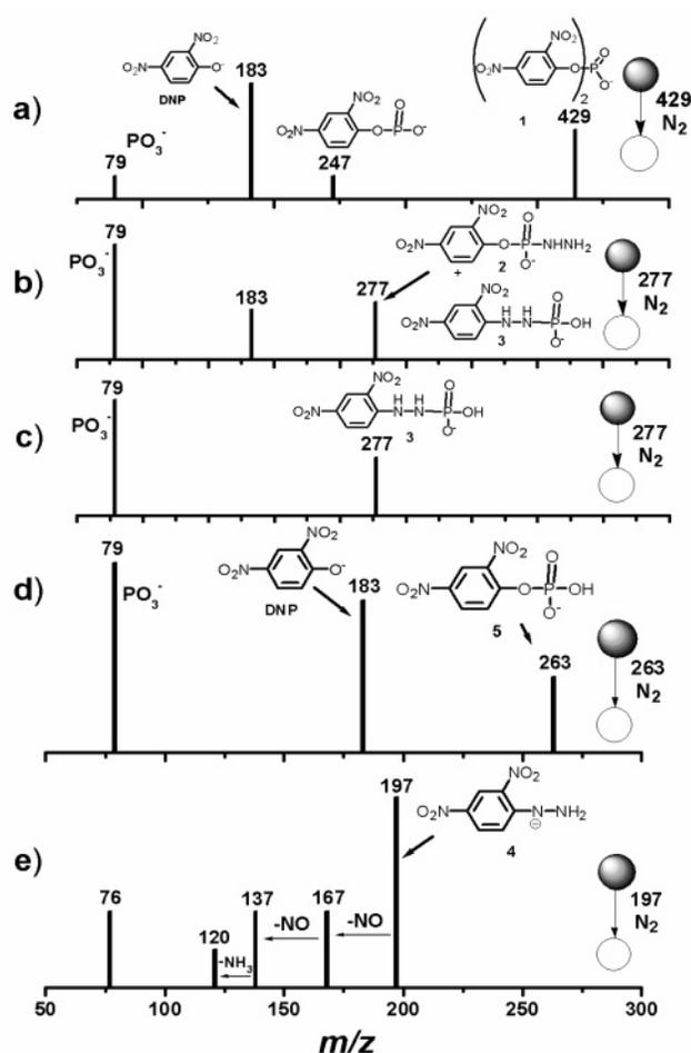
**FIGURE 4.** ESI-MS/MS tandem mass spectra of anionic intermediates observed in the reaction of 0.01 M BDNPP with 0.1 M  $\text{NH}_2\text{NH}_2$  in aqueous methanol (50% v/v) at pH 10. Spectra b and c were taken at 10 and 30 min of reaction, respectively.
