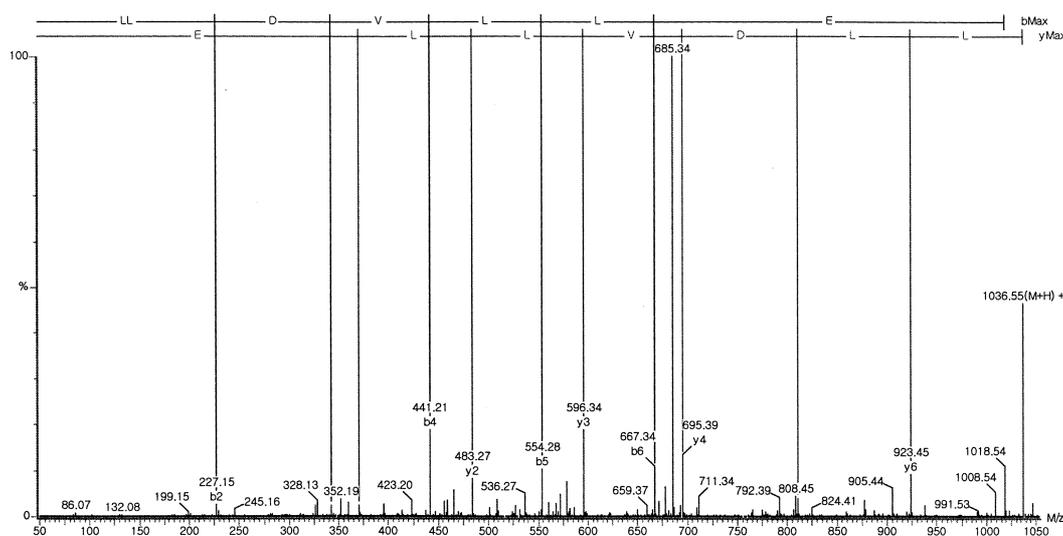
**Fig. 3.** ESI-MS/MS spectrum of the protonated molecule of  $m/z$  1036. The fragment ions (with the corresponding amino acid residues) are marked by dashed lines.
