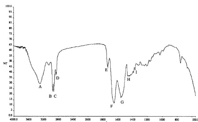
**Fig. 1.** Infrared spectrum of the surfactant obtained from cassava wastewater. Letters represent the bands explained on text.
