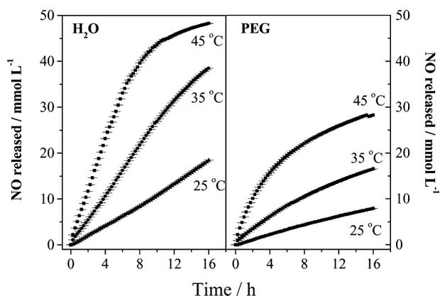
Fig. 3. Kinetic curves of NO release from GSNO ( $46.5 \text{ mmol L}^{-1}$ ) in aqueous solution and in PEG matrix in the dark at 25, 35, and 45 °C. The increases in the concentration of NO were calculated from the corresponding decomposition curves monitored at 545 nm (for details see Experimental procedure).
