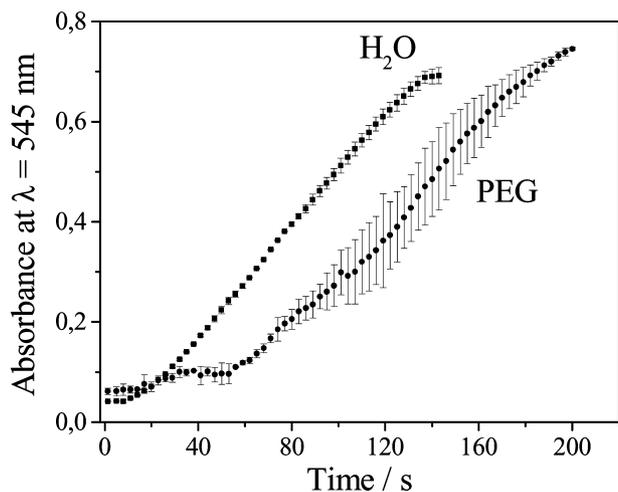
Fig. 2. Kinetic curves monitored at 545 nm corresponding to the synthesis of GSNO by bubbling a gaseous NO/synthetic air mixture through GSH (46.5 mmol L<sup>-1</sup>) in aqueous solution and in PEG matrix, as indicated in the figure.
