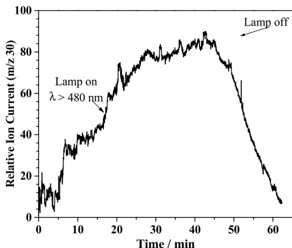
Fig. 8. Real time monitoring of the  $m/z$  30 ( $^{14}\text{N}^{16}\text{O}^+$ ) ion current from the headspace of 500  $\mu\text{L}$  PEG/ $\text{H}_2\text{O}$ -GSNO solution containing 46.5  $\text{mmol L}^{-1}$  of GSNO at 25  $^\circ\text{C}$  under irradiation with  $\lambda > 480$  nm.
