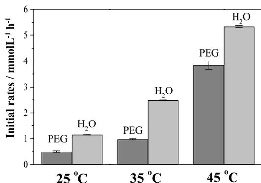
Fig. 4. Initial rates of NO release from GSNO ( $46.5 \text{ mmol L}^{-1}$ ) in aqueous solution and in PEG in the dark at 25, 35, and 45 °C. Rates were calculated from the kinetics curves of Fig. 3.
