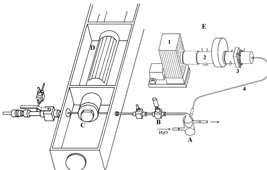
Fig. 1. System used for MS detection of free NO in the nearly air-free headspace of liquid PEG and PEG-GSNO solutions. (A) Thermostated ampoule containing the samples; (B) needle valve; (C) EI ion source of the mass spectrometer; (D) high-transmission 3/4 in. mass analyzer quadrupole; and (E) Irradiation system: (1) mercury-arc lamp, (2) water filter, (3) holder for optical glass filter, and (4) liquid light guide.
