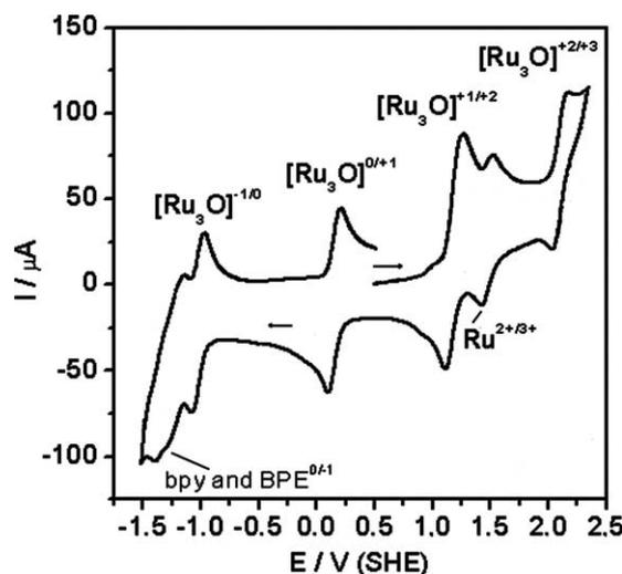
Fig. 5. Cyclic voltammogram of the  $[\text{Ru}(\text{bpy})_2(\text{BPE})_2\{\text{Ru}_3\text{O}(\text{CH}_3\text{COO})_6(\text{py})_2\}_2](\text{PF}_6)_4$  complex in  $3 \times 10^{-3} \text{ mol l}$  acetonitrile solutions,  $0.1 \text{ mol l}$  TEAP, room temperature, scan rate =  $200 \text{ mV s}^{-1}$ .
