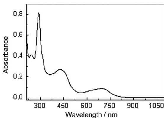
Fig. 4. Absorption spectrum of the  $[\text{Ru}(\text{bpy})_2(\text{BPE})_2\{\text{Ru}_3\text{O}(\text{CH}_3\text{COO})_6(\text{py})_2\}_2](\text{PF}_6)_4$  complex, in acetonitrile solution.
