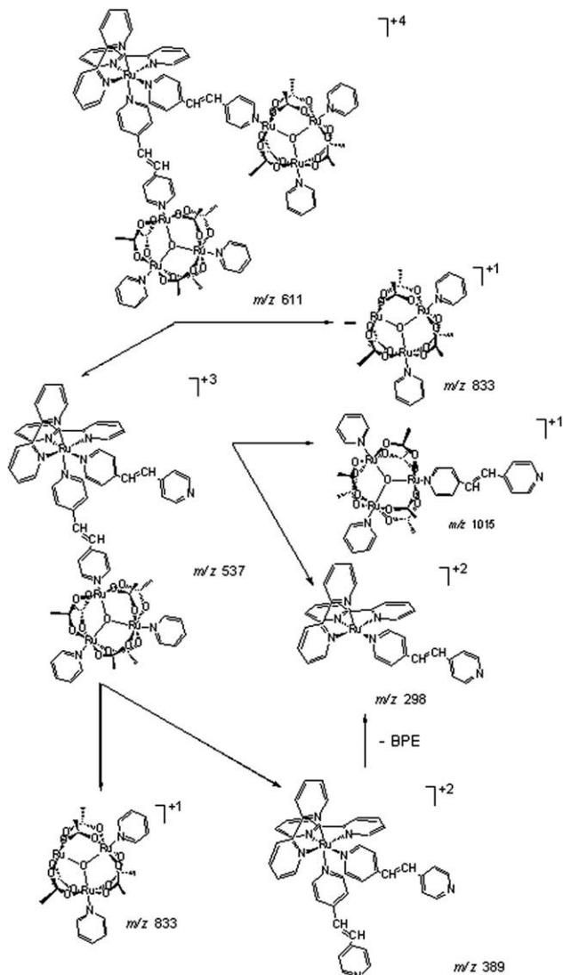
Fig. 3. Dissociation routes for the 15 eV collision-induced dissociation of gaseous  $[\text{Ru}(\text{bpy})_2(\text{BPE})_2\{\text{Ru}_3\text{O}(\text{CH}_3\text{COO})_6(\text{py})_2\}_2]^{4+}$  ions.
