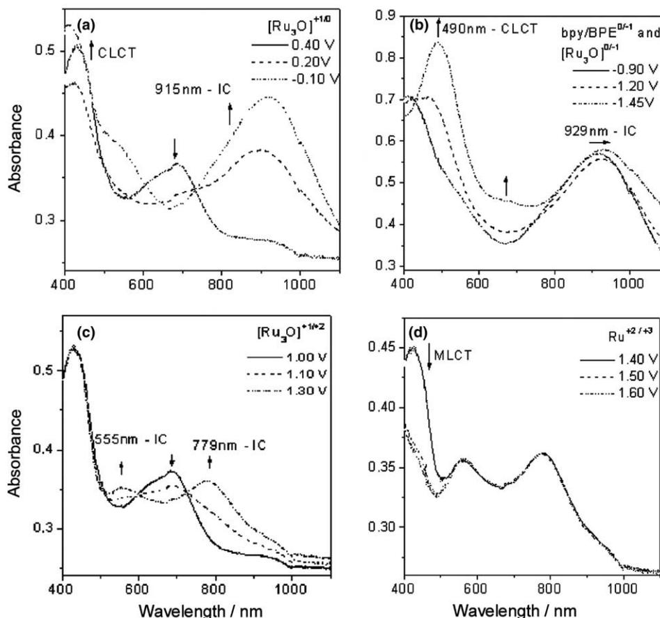
Fig. 6. Spectroelectrochemical behavior of  $[\text{Ru}(\text{bpy})_2(\text{BPE})_2\{\text{Ru}_3\text{O}(\text{CH}_3\text{COO})_6(\text{py})_2\}_2](\text{PF}_6)_4$  in  $3 \times 10^{-3}$  mol/l acetonitrile solutions, 0.1 mol/l TEAP, as a function of the applied potentials.
