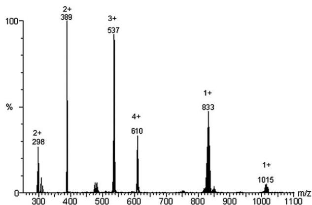
Fig. 2. ESI tandem mass spectrum for 15 eV collision-induced dissociation of  $[\text{Ru}(\text{bpy})_2(\text{BPE})_2\{\text{Ru}_3\text{O}(\text{CH}_3\text{COO})_6(\text{py})_2\}_2]^{4+}$  ions ( $m/z$  610). The charge states for the ions are indicated.
