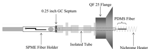
**Fig. 1** Schematic of sample preconcentration and inlet system. The SPME fiber is introduced through a GC septum into the vacuum system via a series of swagelok connectors coupled to a QF25 vacuum flange. An isolated 1/16 inch od stainless steel tube was held at an elevated potential to allow resistive heating of a nichrome wire to heat the PDMS and desorb accumulated analyte.
