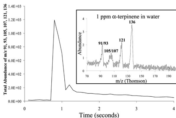
**Fig. 5** Multiple ion monitoring trace of headspace sampling (5 min) of 1 ppm  $\alpha$ -terpinene. The system has a 10–90% rise time of 0.1 s and 90–10% fall time is 1.2 s. A full mass spectrum of 1 ppm  $\alpha$ -terpinene is shown in the inset.
