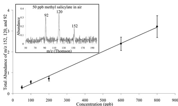
**Fig. 2** Total abundances of characteristic ions of methyl salicylate ( $m/z$  152, 120, and 92) as a function of methyl salicylate in air concentration. Note the linear response ( $y = 0.0039x + 0.0669$ ,  $R^2 = 0.9954$ ) which is maintained from the limit of detection, 25 ppb, up to 800 ppb. A mass spectrum of 50 ppb methyl salicylate in air is shown in the inset.
