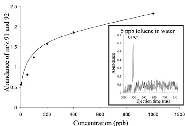
**Fig. 4** Analytical performance when sampling headspace over aqueous toluene solutions. Limit of detection is 1 ppb with 5 min exposure. Linearity of response ( $y = 0.005x + 0.5672$ ,  $R^2$  value of 0.9996) occurs from concentrations corresponding to the limit of detection up to 200 ppb. A mass spectrum of 5 ppb toluene sample is shown in the inset.
