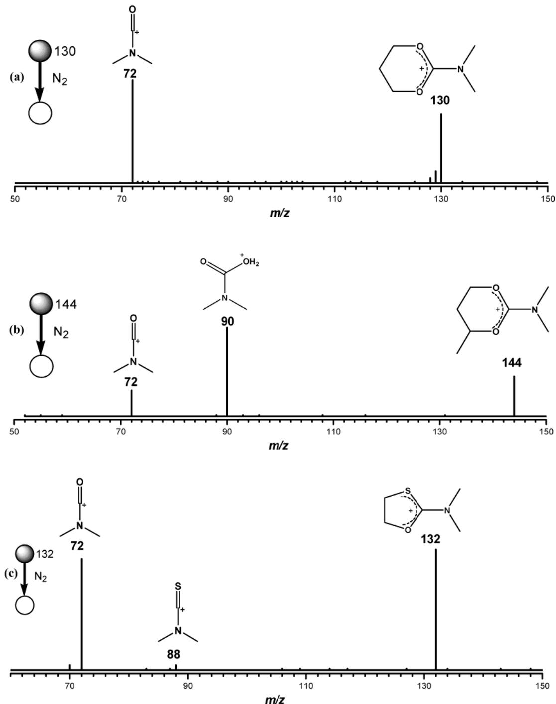
Figure 4. Tandem ( $MS^2$ ) product ion mass spectra for low-energy CID of the cyclic ionic acetals formed by APCI in-source transacetalization of the acylium ion with (a) 1,3-dioxane, (b) 4-methyl-1,3-dioxane, and (c) 1,3-thioxolane.
