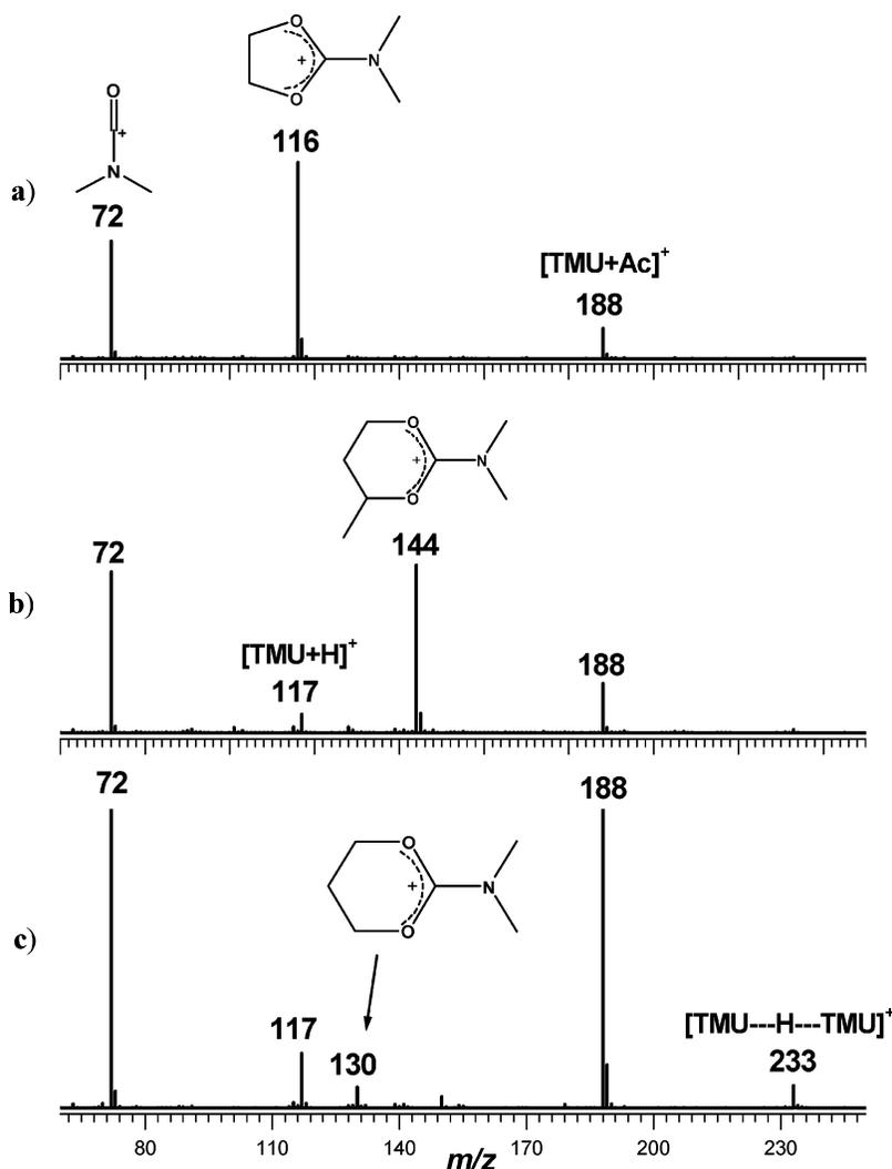
Figure 2. APCI in-source IMR mass spectrum in water/methanol solutions of the acetal (a) **1**, (b) **2**, and (c) **3** with the addition of TMU for in-source generation of the acylium ion  $(\text{CH}_3)_2\text{NCO}^+$  ( $\text{Ac}^+$ ). Note that the TMU background ions were not subtracted.
