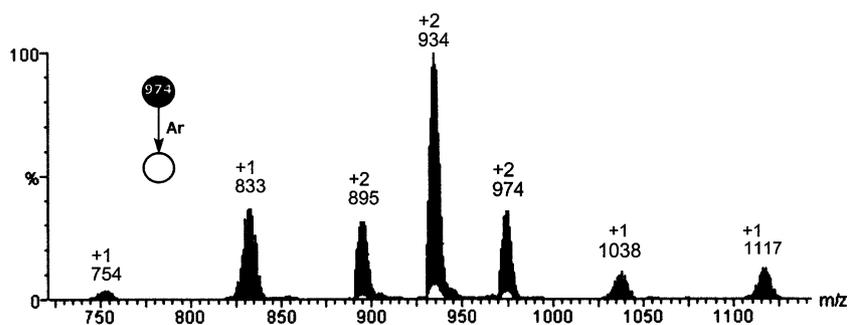
Fig. 4. Tandem product ion mass spectrum for the mass-selected ionic cluster of  $[\{\text{Ru}_3\text{O}(\text{CH}_3\text{COO})_6(\text{py})_2\}_2(\text{BPEB})]^{2+}$  centered at  $m/z$  974. The ion shows a structural diagnostic dissociation behavior with characteristic charge splitting and ligand loss dissociation (see Scheme 1). Singly (+1) and doubly (+2) charged ions are labeled.
