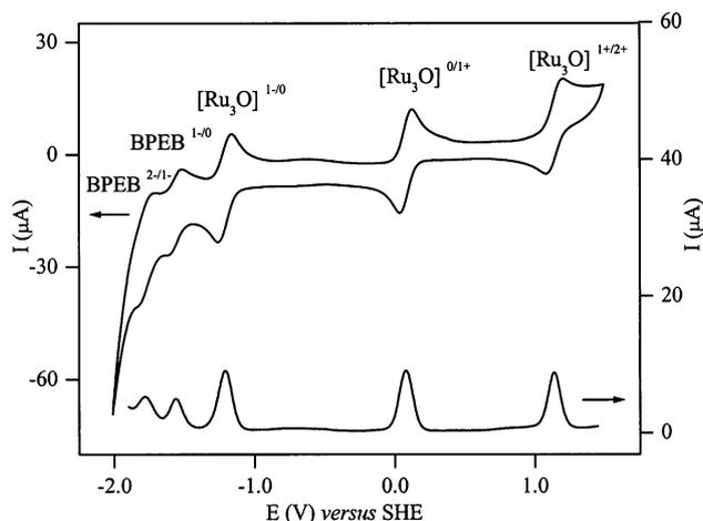
Fig. 7. Cyclic and differential pulse voltammograms of  $[\{\text{Ru}_3\text{O}(\text{CH}_3\text{COO})_6(\text{py})_2\}_2(\text{BPEB})(\text{PF}_6)_2]$  dimer in DMF,  $0.1 \text{ mol dm}^{-3}$  TBAPF<sub>6</sub> solution, at room temperature.
