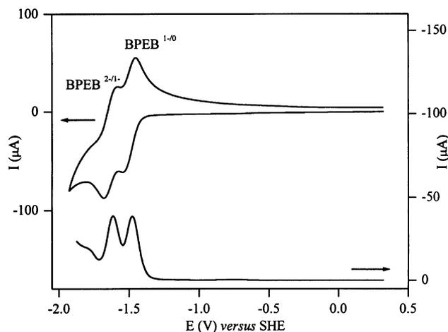
Fig. 5. Cyclic and differential pulse voltammograms of the BPEB free ligand in DMF,  $0.1 \text{ mol dm}^{-3}$  TBAPF<sub>6</sub> solution, at room temperature.
