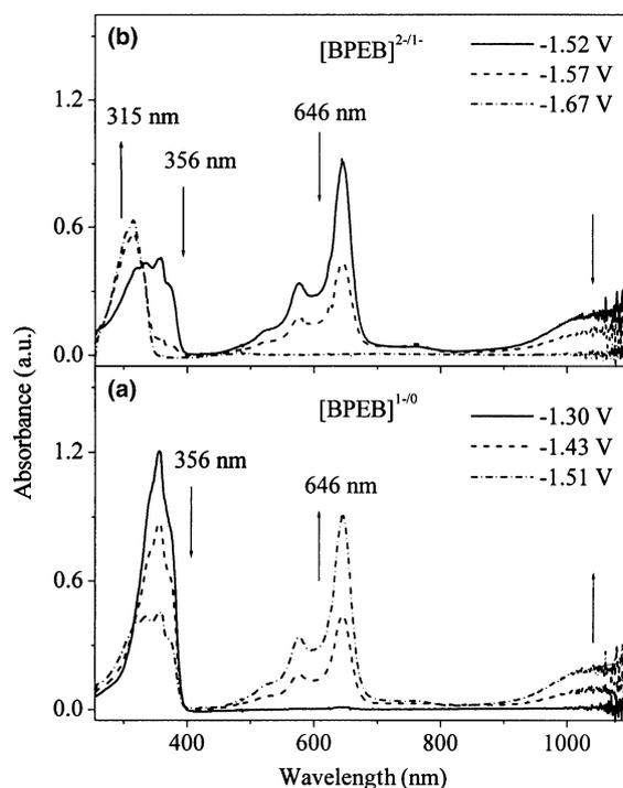
Fig. 6. Spectroelectrochemical behavior of the BPEB bridging ligand in DMF solution; the potential ranges and the assignment of the redox processes are indicated in the figure.
