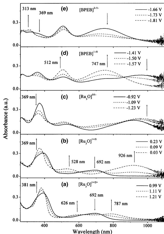
Fig. 8. Spectroelectrochemical behavior of the dimer  $[\{\text{Ru}_3\text{O}(\text{CH}_3\text{COO})_6(\text{py})_2\}_2(\text{BPEB})](\text{PF}_6)_2$  in DMF solution; the potential ranges and the tentative assignment of the redox processes are indicated in the figure.
